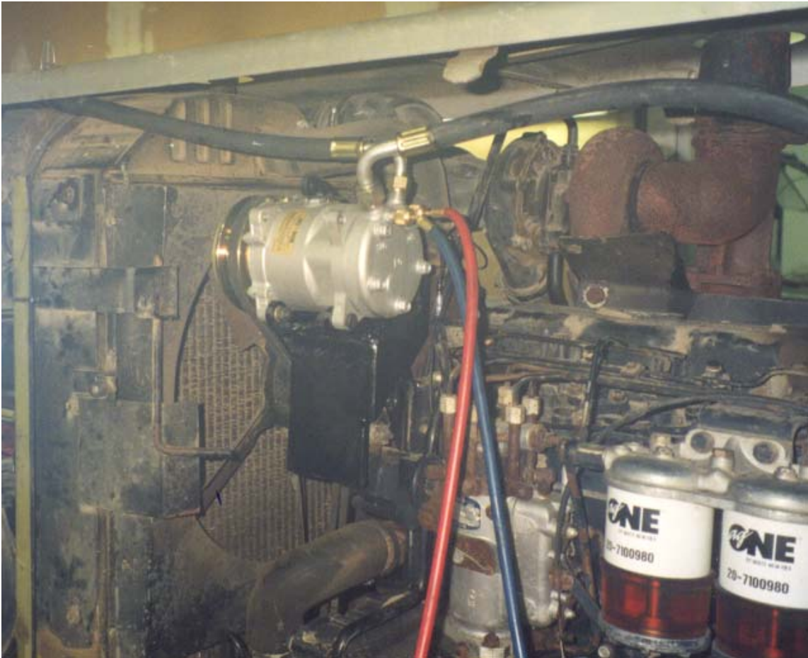
Compressor and mount in place on engine.
